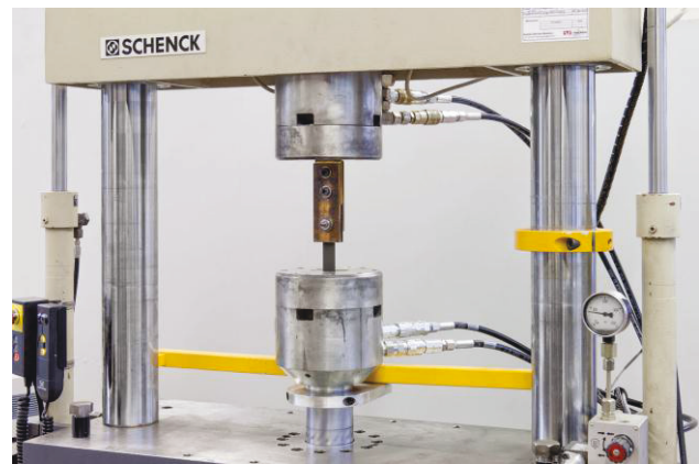
FIG 20. LCF testing of plane test coupon at NLR
