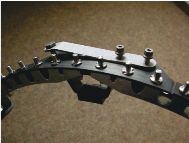
FIG 4. Former Composite Hybrid Unison Ring designed by DLR Stuttgart combining composites and metal
