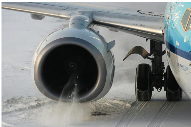
FIG 6. At the Boeing 737 the installation of the engines below the wings already at the older models required advanced, adopted pylon- and nacelle design
