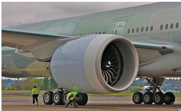
FIG 5.above.Fan-tip speed, ground clearance of engines and drag-effective wetted area of enlarged nacelles becomes a performance and safety issue with increasing by pass ratio thus fan diameter of the engine
