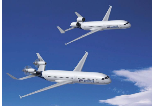
Fig 16. Placing the Open-Rotor engines beside each other, in a way similar to turbofan engines, can result in a dangerous scenario where in the case of a Rotor Burst the functioning engine gets damaged by the failed engine [13].
