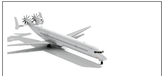
Fig15. Example of a proposed aircraft concept using the open-rotor engine architecture with aft mounted engines in questionable side by side arrangement [12].
