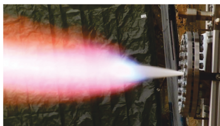
FIG 13. Test # 3 Oxygen Excess
