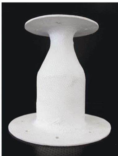
FIG 6. OCMC Rocket Engine Prototype [7]
