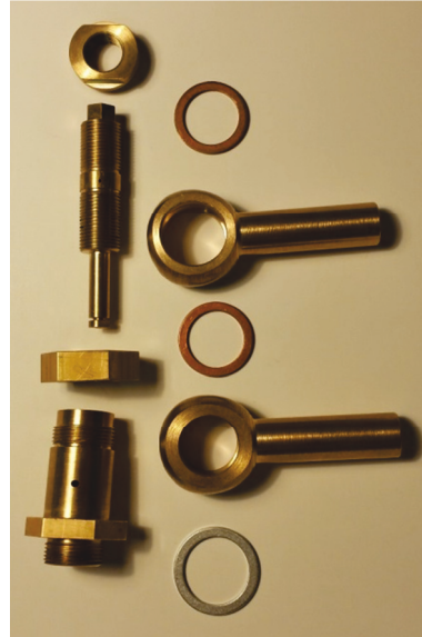
FIG 5. Coaxial Test Injector in Parts [6]
