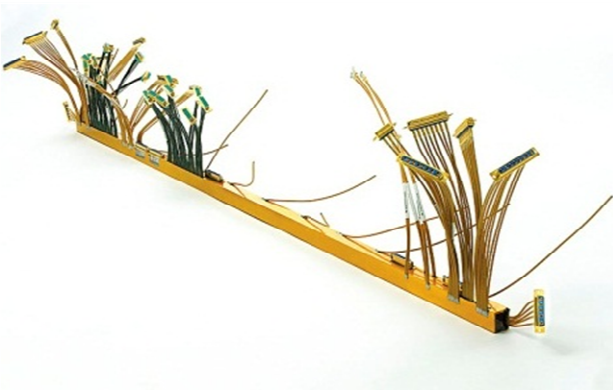
PICTURE 9. Monolayer Bar Type E with flexible connection links.
