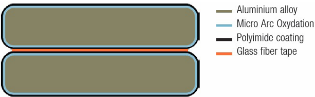
PICTURE 8. Double layer bar (Type II) for the link between high power battery parts.
