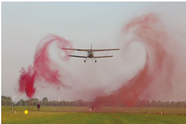
FIG 12. Wake roll-up of the An-2 visualised by smoke
