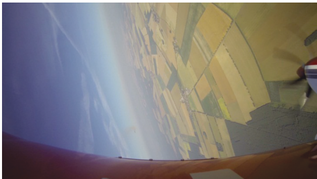
FIG 13. DR 400 wing view at maximum bank angle after an encounter into an An-2 wake
