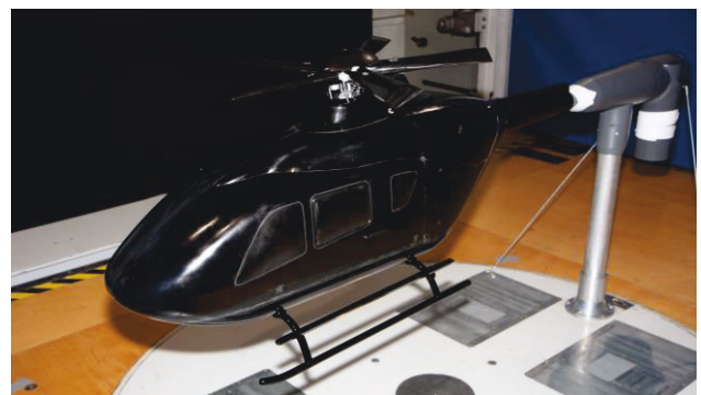
Fig.1. Baseline configuration, TEL-class helicopter fuselage with rotating rotor head
