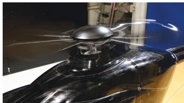
Fig.4. Rotating model rotor head
