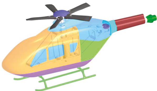
Fig.2. Modular design of the wind tunnel model
