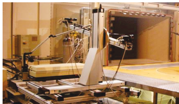
Fig.5. Stereo PIV system
