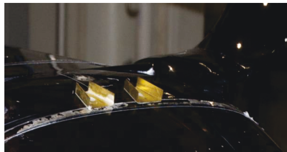
Fig.16. Belly mounted vortex generator pair
