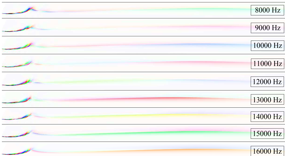
FIGURE 17: Modes of the heat release rate fluctuations in the near and far zone, each with the frequency equal to excitation frequency at LP3.
