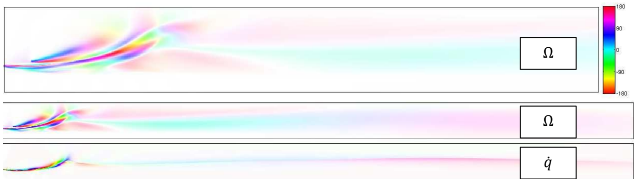
FIGURE 15: Mode of the vorticity fluctuations in the near and far zone (top/middle) compared to the mode of the heat release fluctuations, with the frequency equal to the excitation frequency at LP3 with 11 000 Hz acoustic forcing.
