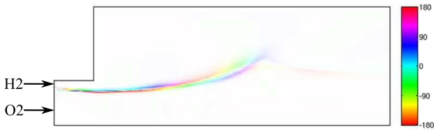
FIGURE 11: Mode of the heat release fluctuations in the near zone, with the frequency equal to excitation frequency at LP3 with 11000 Hz acoustic forcing.
