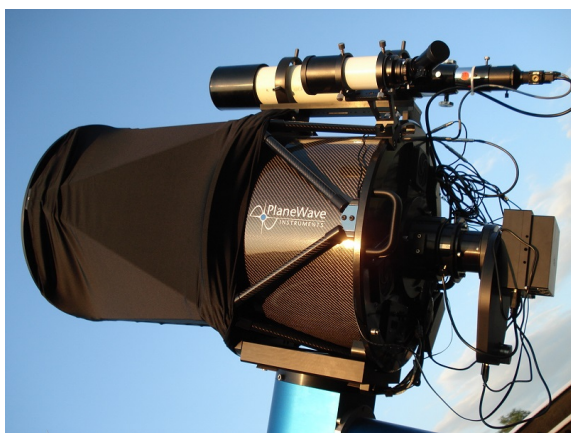
Figure 2: The passive optical set-up as of July 2013. The main telescope is the Planewave CDK 17" described in the text, the two smaller telescopes are so far only used for calibration and tests. The light from the main telescope is recorded by an FLI ProLine camera equipped with a 7-slot filter wheel.
