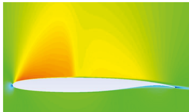
Figure 8 Distribution of the Mach number around a 9% supercritical airfoil
