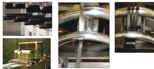
FIG 6: Manufacturing of carbon-fibre – steel-fibre hybrid material by filament winding
