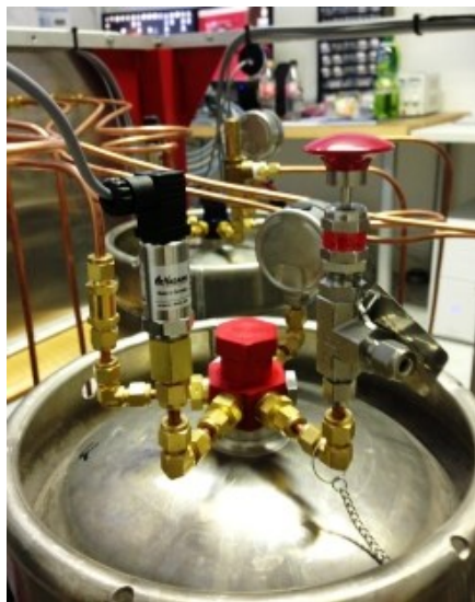
FIG 4 – The adapter for the ethanol tank with the mounted instruments and the LOX tank adapter in the background.
