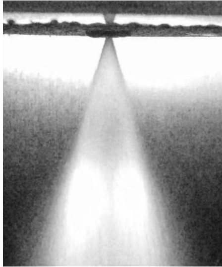
FIG 9 – Spray cone of the LOX nozzle
