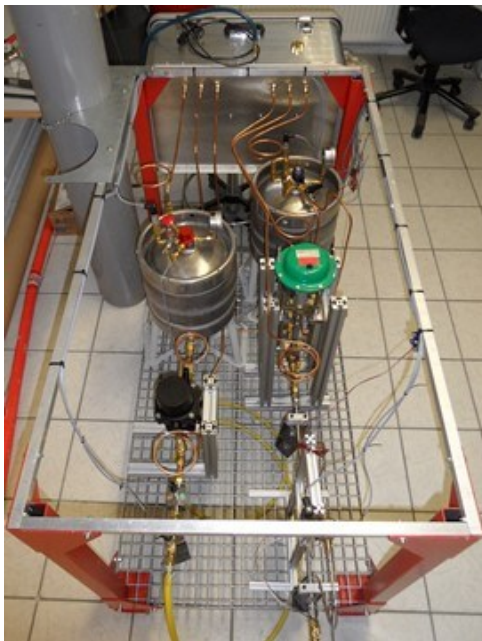
FIG 2 – Test bench with ethanol (left) and LOX pipeline (right)
