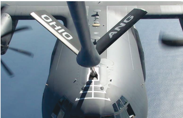
FIG. 7. UARRSI with aerial refueling boom 1
