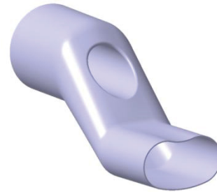
FIGURE 16. Generic inlet concept for aerodynamic analysis
