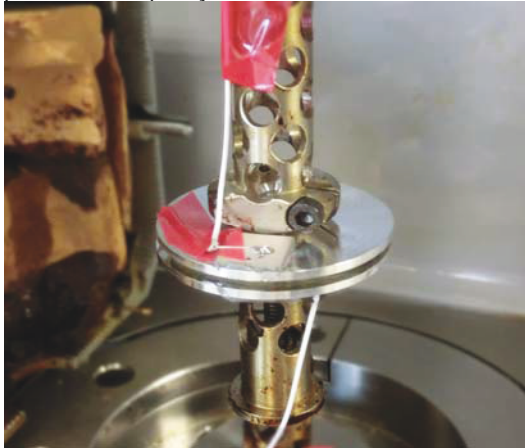
Fig. 12: Piezoceramis integrated into rheometer
