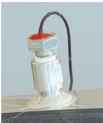
Fig. 2: Integration of ultrasound transducer in vacuum bagging
