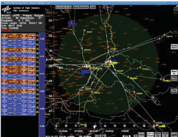
Figure 4 Traffic Scenario with arrival and departure traffic for airport LKPR negotiated with an arrival planning tool
