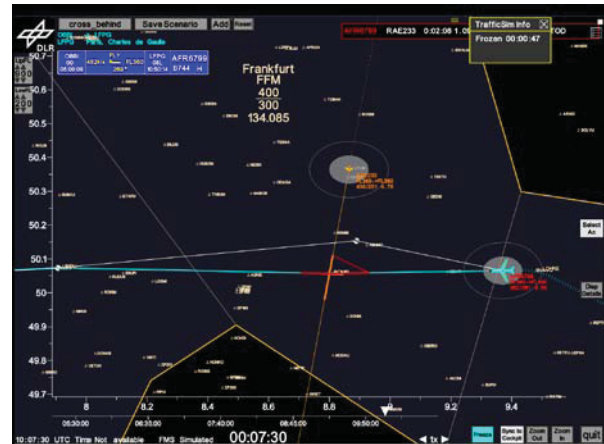
Figure 8 A conflict situation and advisory to solve the conflict shown in TrafficSim.
