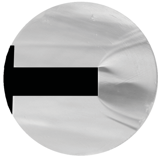
Figure 16. Schlieren image with jet and surrounding flow ( p_{t,SC} = 16.13 bar, T_{SC} = 470 K and Ma_e = 2.5 , p_{t,\infty} = 16.79 bar, T_\infty = 470 K and Ma_\infty = 5.9 , top: single image bottom: averaged image).
