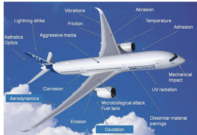
FIGURE1: Main requirements on surface protection system
